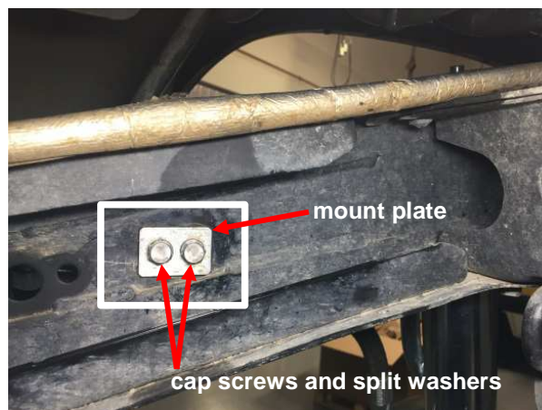
Looking at inside of frame rail
