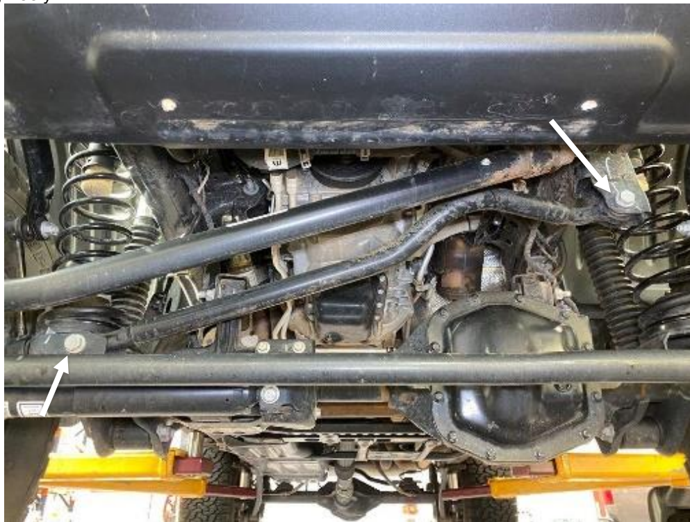
Track Bar Bolts
