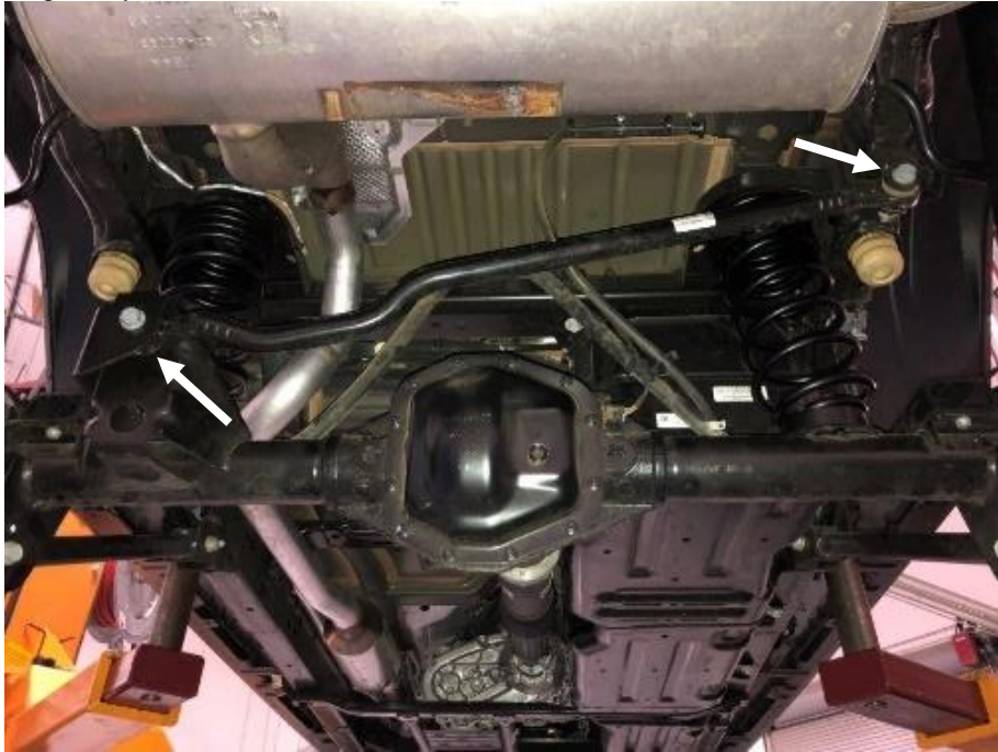
Track Bar Bolts
