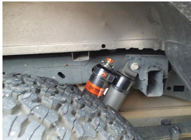
Fig 6: Passenger side rear shock orientation.
