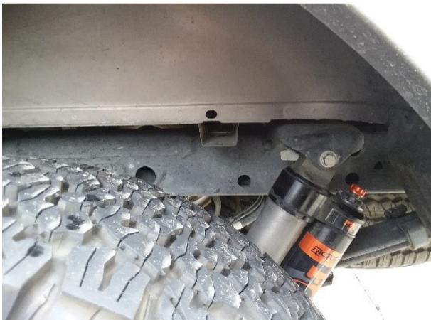
Fig 5: Driver side rear shock orientation.
