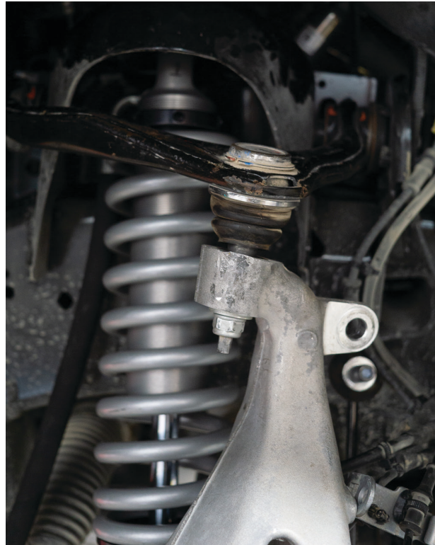
Fig. 14: Reattach UCA to the upright.
