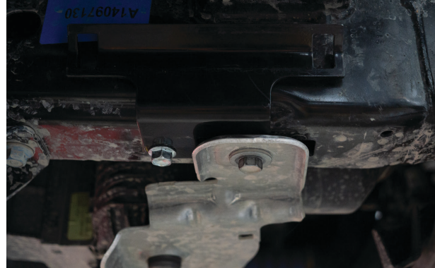
Fig. 9: Install the reservoir bracket.
