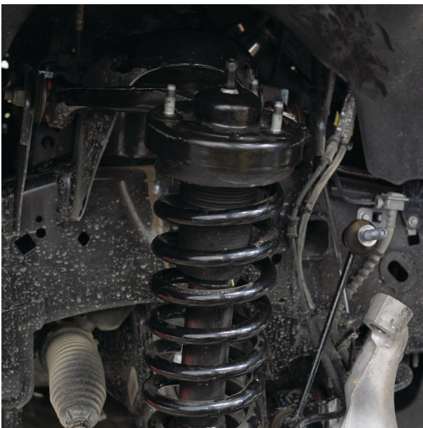
Fig. 6: Free the coil-over.
