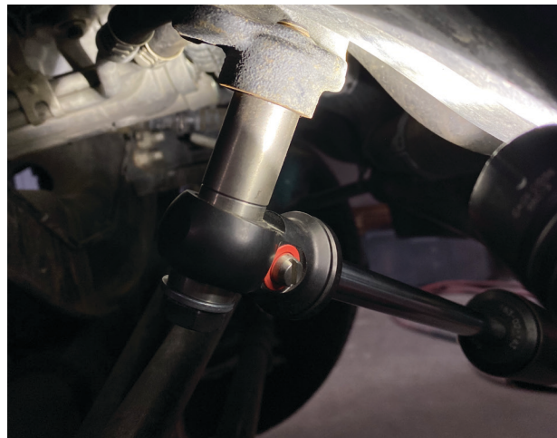
Fig. 1: The adjuster screw on the eyelet is pointed toward the front of the vehicle.
