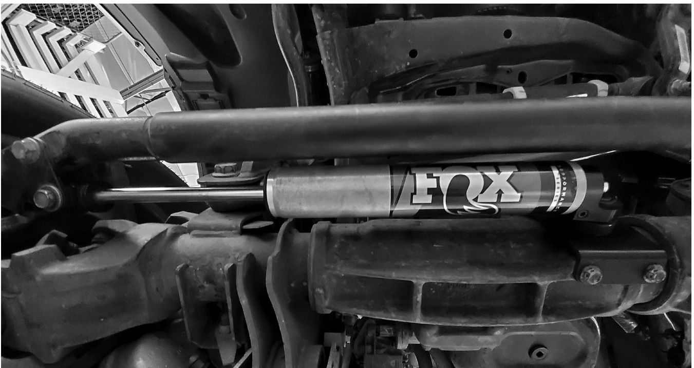
Figure 9: Reasonable shaft clearance
