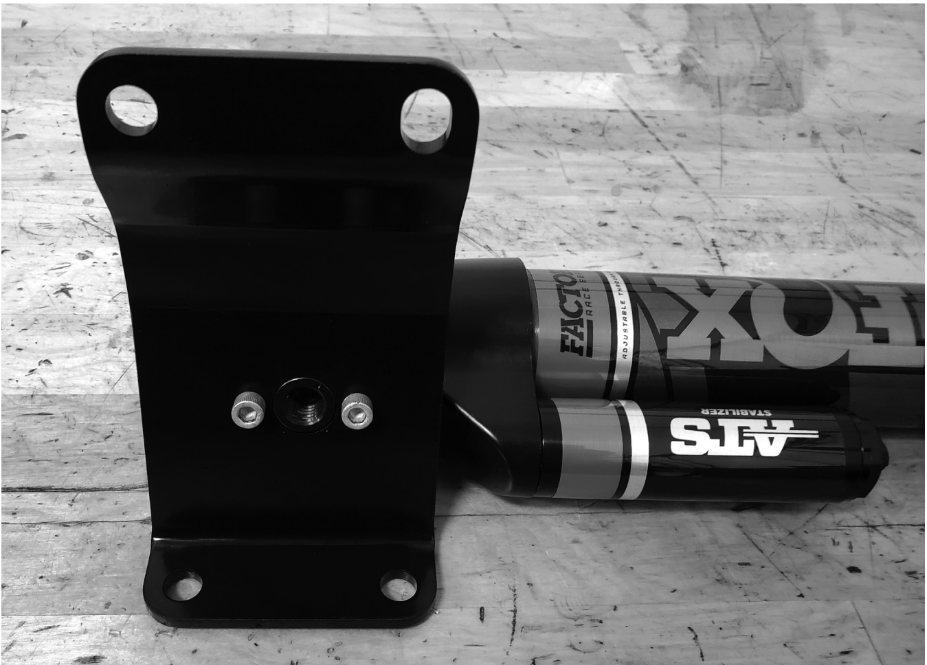
Figure 5: Replacement bracket attached
