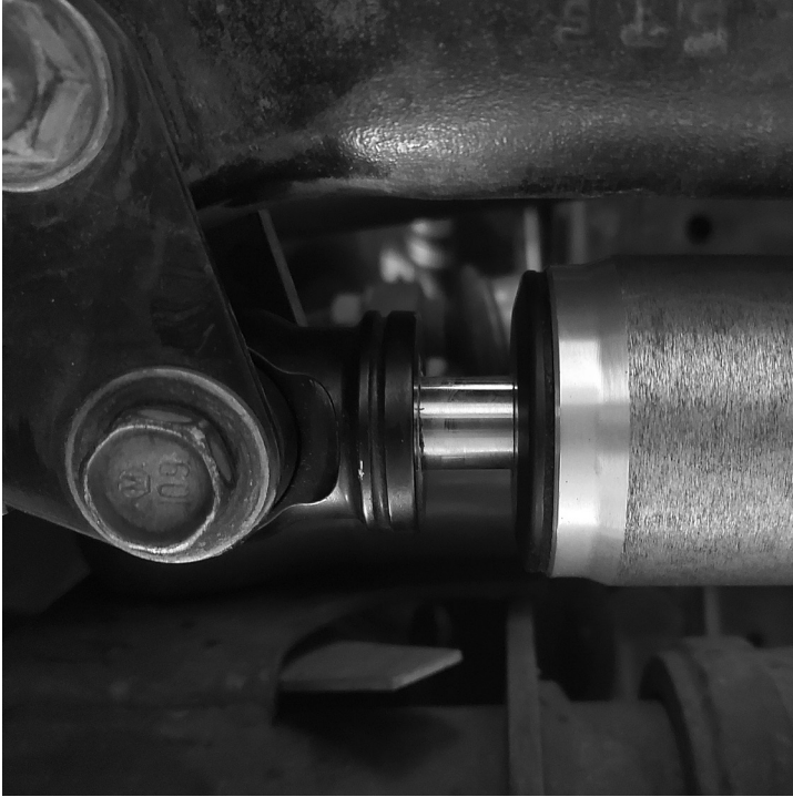
Figure 8: Reasonable shaft clearance
