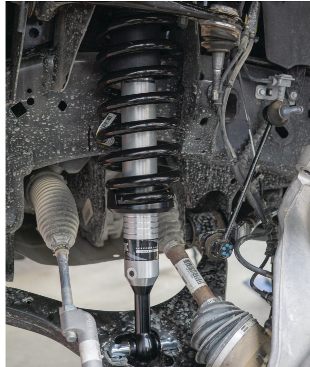
Fig. 15: Install the coil-over.
