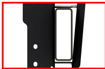
FIGURE C7: View showing an incorrectly tightened inside clamp.
