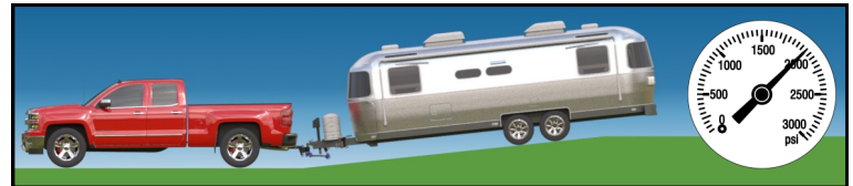
FIGURE L4: Truck and trailer angled up (higher pressure)
